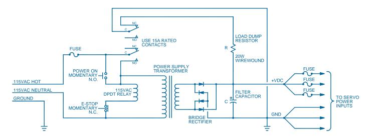
This circuit will quickly bring a servomotor to a stop during an emergency without damaging the motor drives. Snown also is an unregulated power supply though any other type supply may be used as well.
